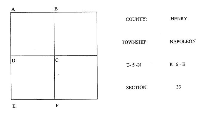
C - Found brick placed vertically over high point of stone. Replaced brick horizontally and placed center punched RR spike over high point. Stone is 16" deep. Pk's 6' north and east.
