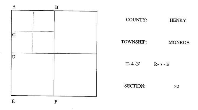
C- Found stone 11" deep. Placed RR spike over same. 45.10' N.E. to 15" tree. 26.58' S.E. to telephone pole. (GONE) 142.12' S.E. to power pole. (duplex e/s)
