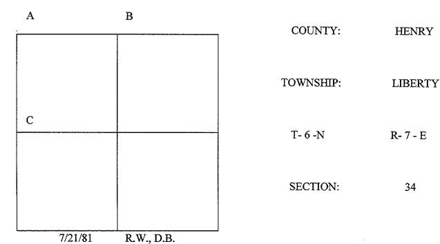
A - Found stone (7"x8"x25") 15" below road surface. Placed center punched RR spike on surface over high point of stone. Pk's 6' south and west. Stone is 9.6' south of north edge 20' pavement and 6.0' east of west edge 18' pavement.
