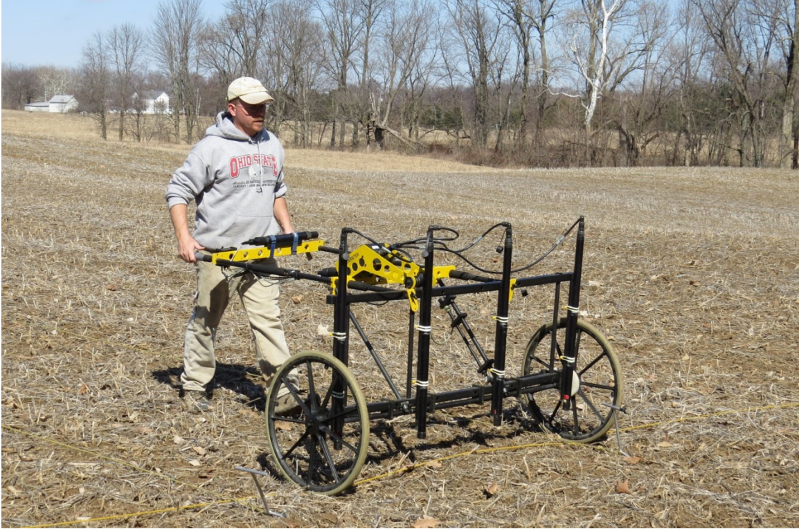
Figure 2. Geophysical instrument used during the survey work: a Foerster Ferex 4.032 DLG 4-probe fluxgate gradiometer.
